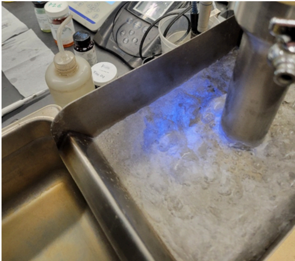
Figure 5: A photo showing the floatation testing with scheelite illuminated by ultra-violet light. Initial floatation testing returned an 84.7% recovery for tungsten from the Rhosgobel deposit.
